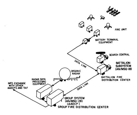
Figure 3. Fire distribution system AN/MSG-4 (Missile Monitor).
