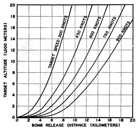
Figure 25. Bomb release distance graph (gravity).
