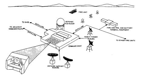
Figure 1. Fire distribution system AN/FSG-1 (Missile Master).
